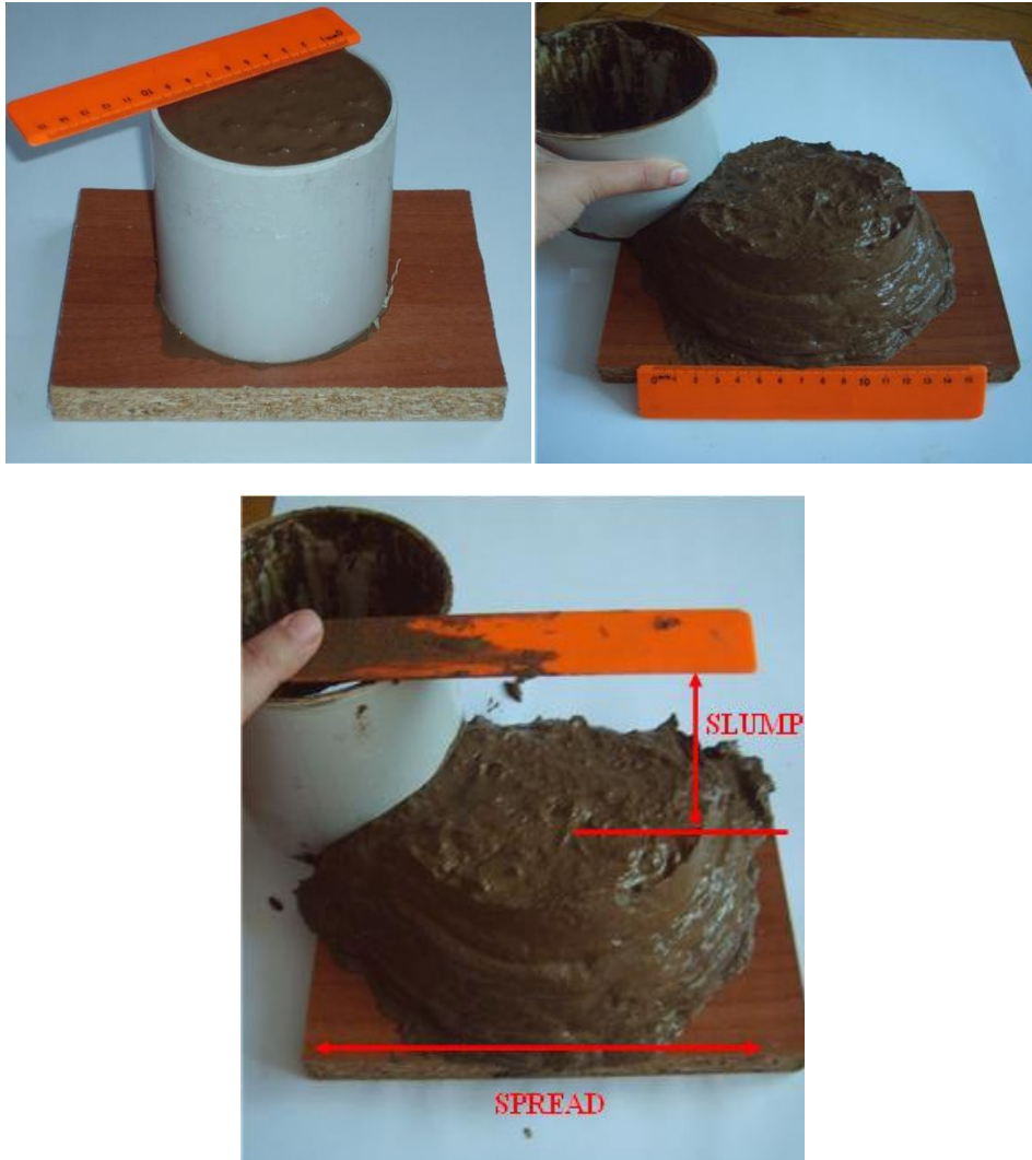
Figure 3. Sequences of slump test application.
